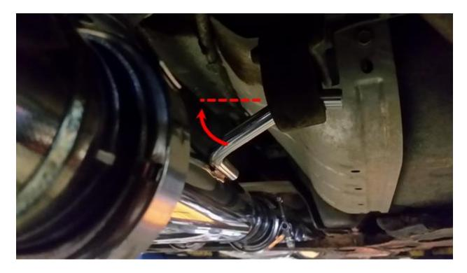
5. Remove the evaporator canister steel heat shield and simply push the thin aluminum heat shield out of the way as needed (the heat shield is only needed for the stock exhaust). \*NOTE: If the heat shield is not removed the exhaust tube will contact the edge of the heat shield and it will not fit properly, possibly causing damage to the bumper.
