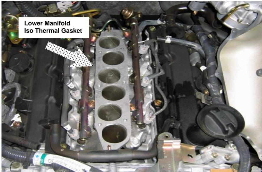
If you are installing a MREV2, first clean it of any dust or debris, then replace the old lower collector with the MREV2. Verify correct orientation of the gasket when it is placed on the intake manifold then install the lower plenum assembly.
