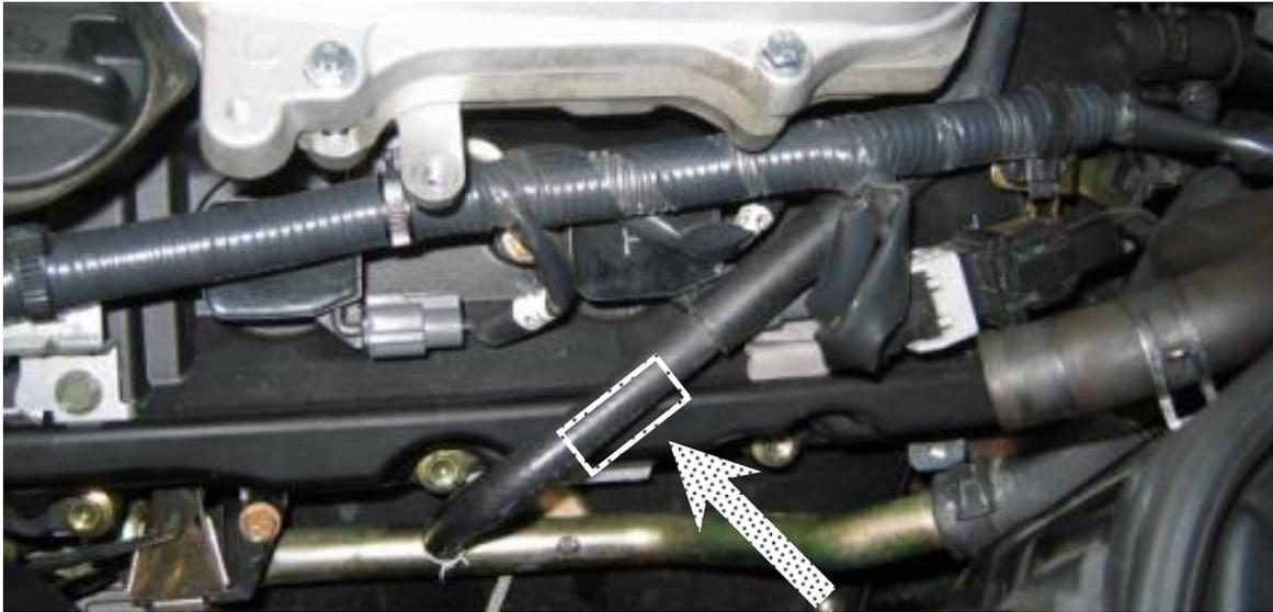
Then install the valve as shown below. The threaded fittings should be sealed with Teflon pipe thread putty or Silicone RTV for a good seal. The pipe threads are tapered and do not need to thread in all the way.
